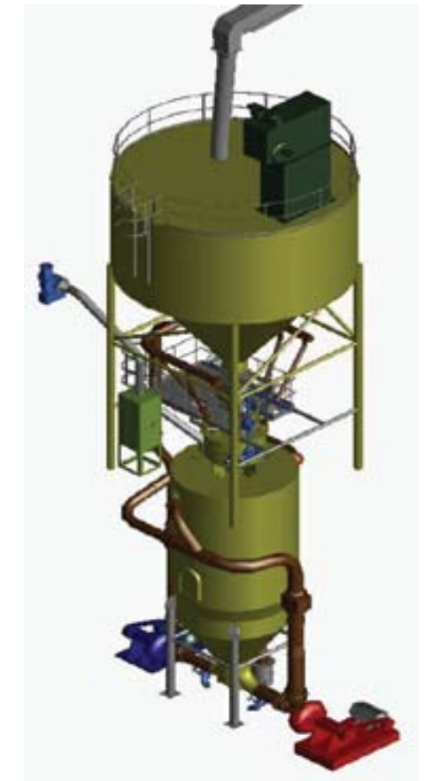
Dense Slurry Mixer Arrangement
